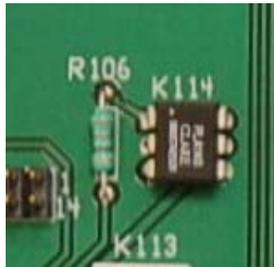
*Note the white dot on K114. Be sure to get the orientation right when you install this component.*
