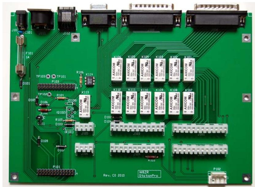
*Note the notch cutouts silkscreened on the rear corners of the main printed circuit board*
