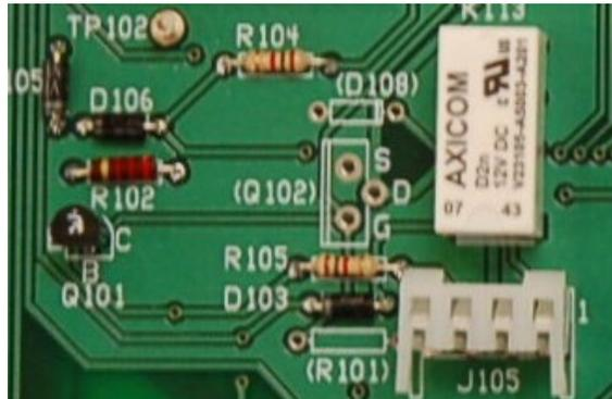
*R101, D108, and Q102 should NOT be installed if the default keying circuit is selected.*
