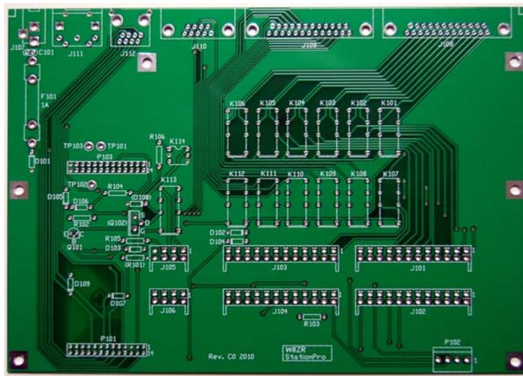
*StationPro Main Circuit Board – Top View*
