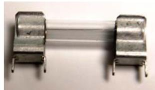
*Insert the 1A fuse into the fuse clips before soldering them to the circuit board.*
